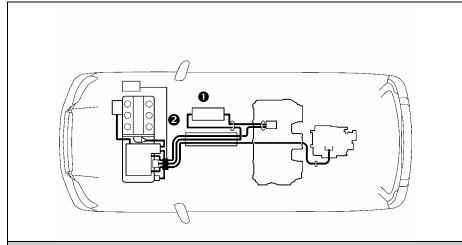
HV Battery and DC-DC Converter Cable Routing
